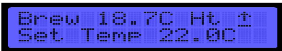
When the heater is on the Heating “Ht” status on the top-right of the main display will change to indicate an up arrow, instead of a single line “\_”. If the buzzer is sounding, this indicates that an alarm has been activated, low or high temperature. The buzzer will also sound briefly any time you press a key.
